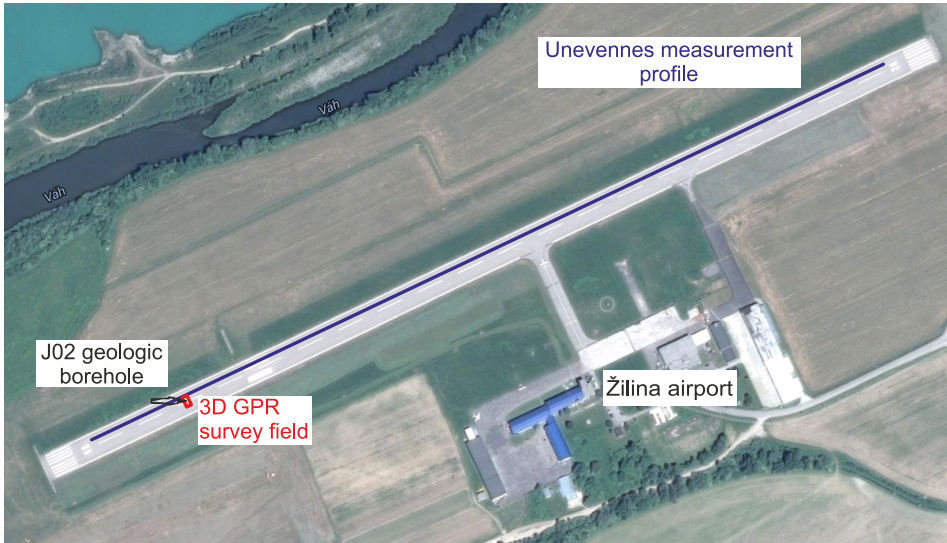
Fig. 1. Satellite map of the Žilina International Airport with the schematic position of the Profilograph GE and GPR measurements.
