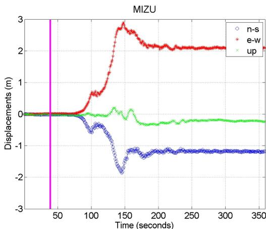
Fig. 1. Coordinate displacements in north-south, east-west and up components on IGS permanent station MIZU during Honshu earthquake 2011, Japan.
