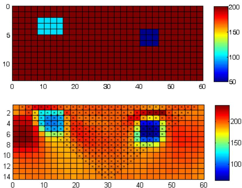
Fig. 1. Comparison between the model data (a) and the inverse image (b) obtained for dipole-dipole electrode configuration in iteration 8 with relative RMS error 2%.
