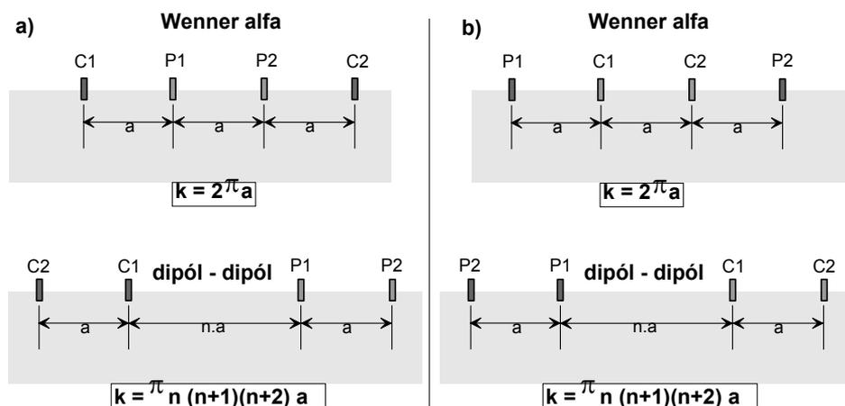
Fig. 1. a) normal position of electrodes, b) reciprocal position of electrodes, C1 and C2 – current electrodes, P1 and P2 – potential electrodes.
