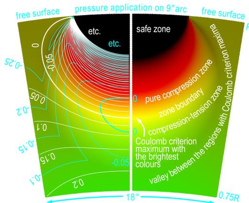
Fig. 1. Detail of the colour map of the stress field near one of the load application regions in Brazilian test.
