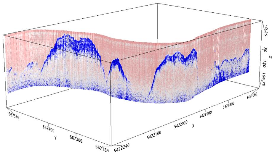
Fig. 1. 3D radargram visualization of the waterborne GPR survey on the Morava River.
