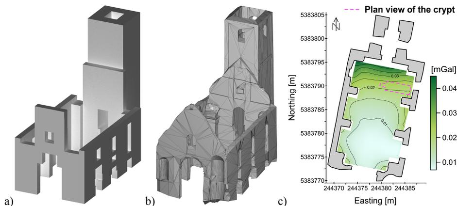
Fig. 1. 3D models of St. Catherine's church ruin (Dechtice) approximated by a set of rectangular prisms – Potent software **(a)** and one polyhedron – PhotoModeler software **(b)**. **(c)** Difference map of corresponding building corrections (model **a** – model **b**).
