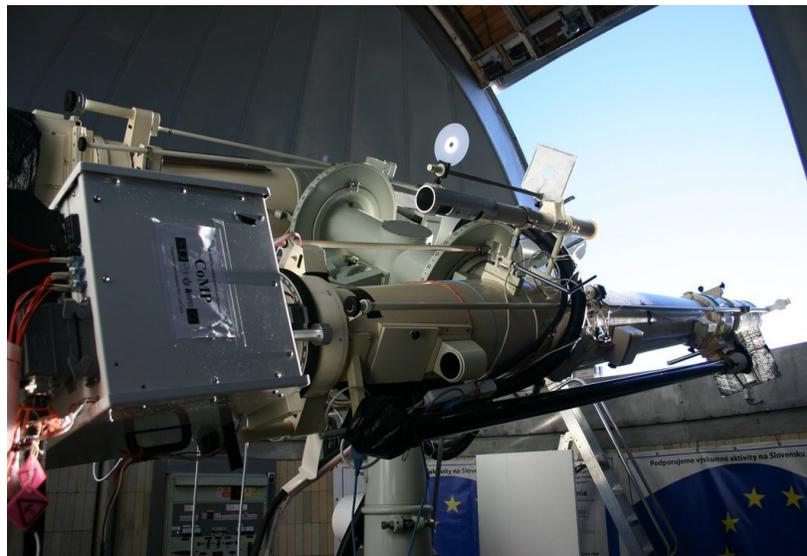
*The CoMP-S and SCD instruments attached to two ZEISS 200/3000 coronagraphs at the Lomnický Štít Observatory.*
