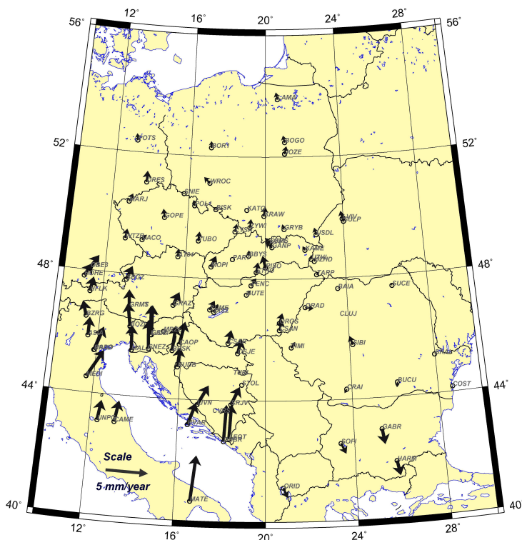
Fig. 1. Intraplate horizontal velocities obtained from long-term GPS monitoring in the region of Central Europe and Balkan Peninsula.
